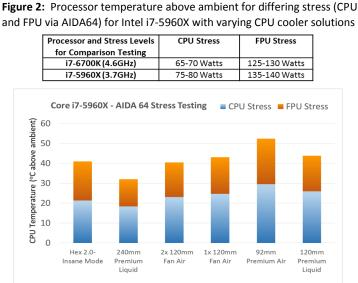
reference. As the data shows, the HEX 2.0 compares very well to the other cooling solutions, but some important features are different on the i7-5960X. First, there is no throttling of the processor with any of the coolers. Second, the temperatures above ambient are much lower although the actual TDP from AIDA64 are higher in both CPU and FPU stress versus the i7-6700K. This is consistent with
